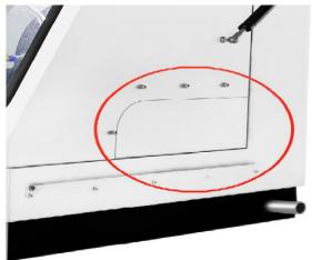
The distance from cutting wheel to left wall is 85mm, from cutting wheel to right side wall is 280mm; If workpieces are very longer, machine right wall reserved hole (loose screen and open the hole will suitable cut off long size samples).
