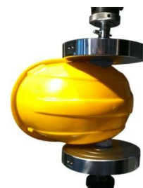
Cyclic test EN 397 Compression Testing Industrial Safety Helmets
