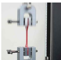
Fatigue Testing on An Elastomer
